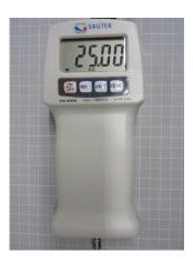
4. The corresponding weight is now attached to the hook. The appliance **must be held still while the weight is attached**; avoid shaking. <u>Tip:</u> hold the device with both hands while both elbows are resting on a table or attach it to a solid object (test bench).
